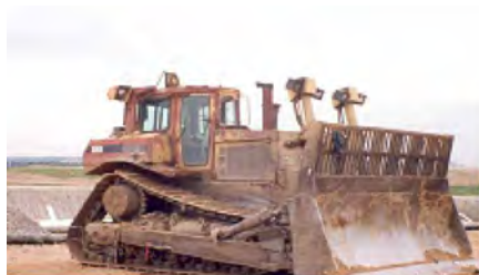
transport and spreading (Bulldozer)
