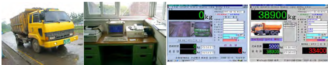
Fig. Annex- 31 Measuring system in the landfill site
