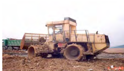
landfilling bulldozer (Compactor)
